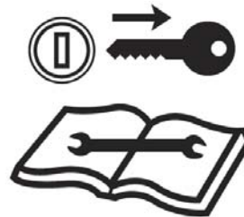
Shut off engine and remove key before performing maintenance or repair work
